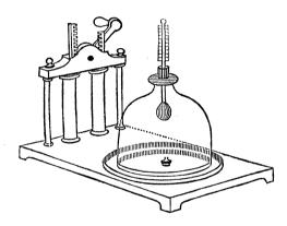
sketch, the plate fitting the receiver air tight when laid upon its open neck), the thermometer sinks rapidly, as the ex-
